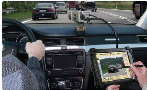
incidents, detect traffic violations, scan license plates, and link to database for real-time information. In addition, the rugged tablet also offers seamless and stable wireless communications so that officers can receive real time information.
